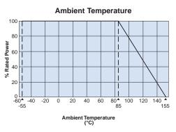
For resistors operated at an ambient temperature of 85°C or above, a power rating shall be derated in accordance with the derating curve.
