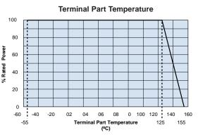
For resistors operated terminal part temperature of described for each size or above, a power rating shall be derated in accordance with the derating curve. Please refer to "Introduction of the derating curve based on the terminal part temperature" in the beginning of our catalog before use.
