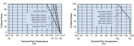
For resistors operated at an ambient temperature of 70°C or above, a power rating shall be derated in accordance with the derating curve. For resistors operated at a terminal part temperature of described for each size or above, a power rating shall be derated in accordance with the derating curve.
