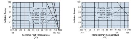
For resistors operated at an ambient temperature of 70°C or above, a power rating shall be derated in accordance with the derating curve. For resistors operated at a terminal part temperature of described for each size or above, a power rating shall be derated in accordance with the derating curve.
