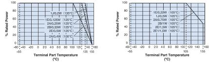
For resistors operated at an ambient temperature of 70°C or above, a power rating shall be derated in accordance with the derating curve.
