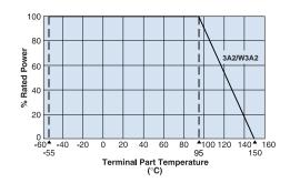
For resistors operated at a terminal part temperature of described for each size or above, a power rating shall be derated in accordance with the derating curve. Please refer to "Introduction of the derating curve based on the terminal part temperature" in the beginning of our catalog before use.
