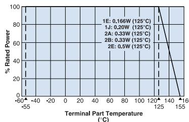
For resistors operated at a terminal part temperature described for each size or above, a power rating shall be derated in accordance with the derating curve.
