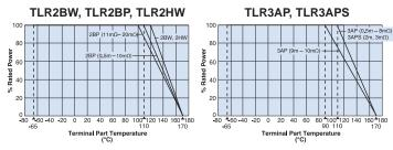
For resistors operated at a terminal part temperature of described for each size or above, a power rating shall be derated in accordance with the derating curve. Please refer to "Introduction of the derating curve based in the terminal part temperature" in the beginning of our catalog before use.
