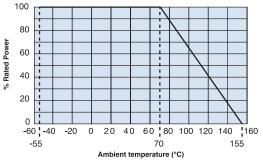
For resistors operated at an ambient temperature of 70°C or higher, the current shall be derated in accordance with the above derating curve.
