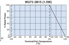
For resistors operated at a terminal part temperature of described for each size or above, the power rating shall be derated in accordance with the derating curve.
